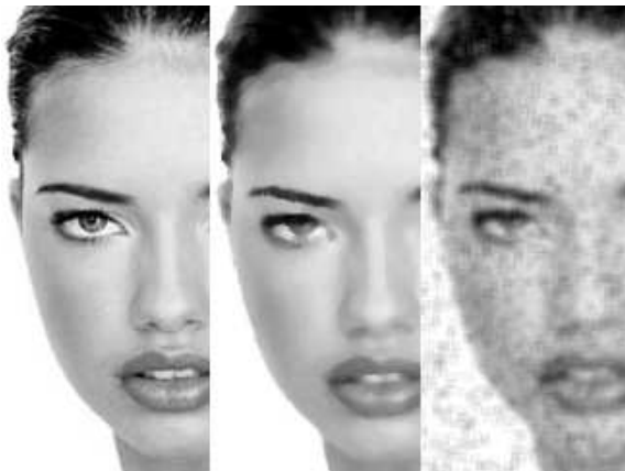
FIGURE: (Enlarged) Noise-free image (left), 5 \times 5 median smoother (center), and 5 \times 5 mean smoother (right).
